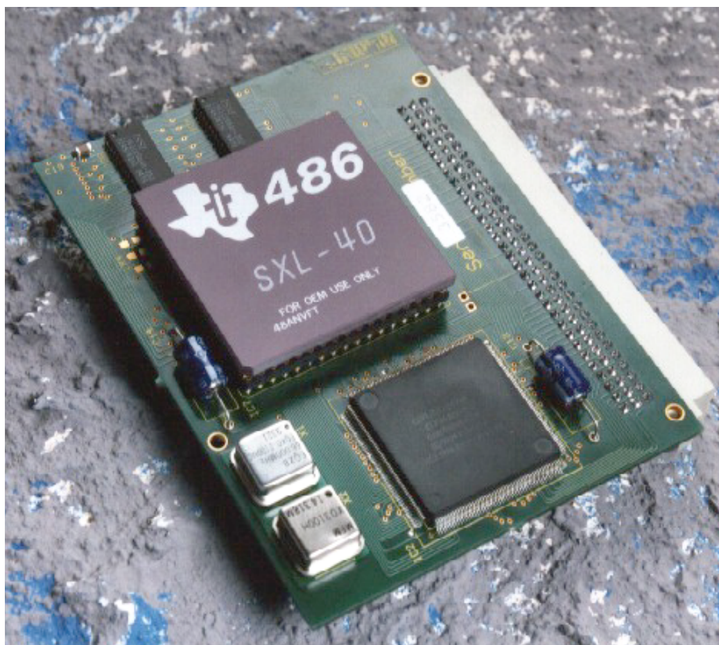
The processor on the PC486 Card tends to get rather hot in use...
